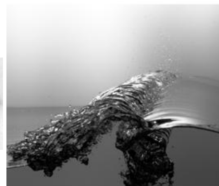
Fragmentation of colliding rims [3] and secondary wave splashing [4]
