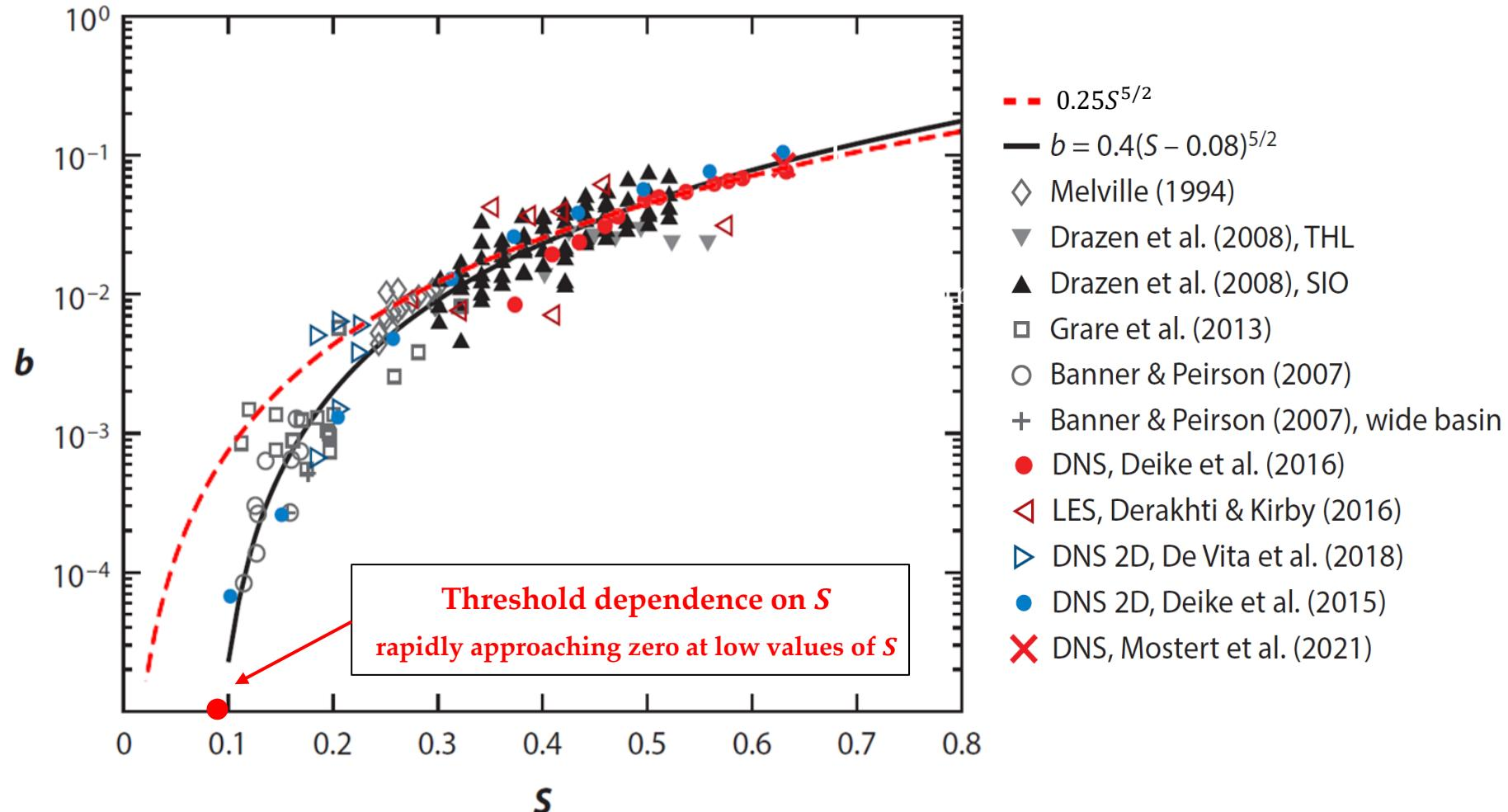
Breaking parameter  $b$  as a function of the wave slope: The inertial scaling of  $b \propto S^{5/2}$  derived by Drazen et al. (2008); and the semi-empirical scaling of  $b \propto (S - S_0)^{5/2}$  by Romero et al. (2012). Data from laboratory observations and numerical results.
