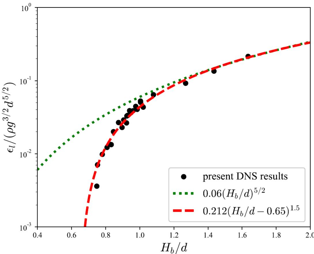
Breaking parameter  $b$  as a function of  $H_b/d$ . Dotted line: inertial scaling of  $b \propto (H_b/d)^{5/2}$ . Dashed line: empirical scaling of  $b \propto (H_b/d - 0.65)^{1.5}$  by introducing a threshold. Data from the present 2D DNS results.
