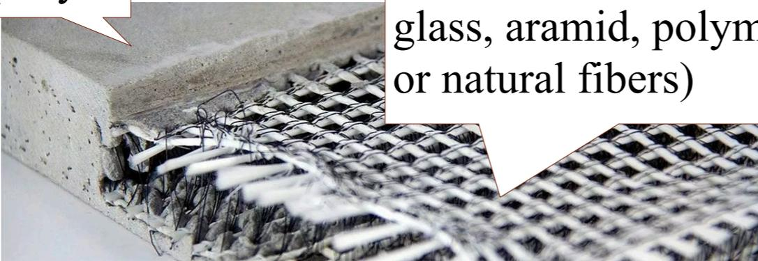
Reinforced matrix (Carbon, glass, aramid, polymer or natural fibers)
