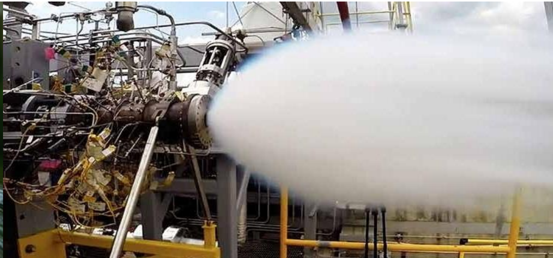
SpaceX raptor engine bipropellant pintle injector cold flow test
